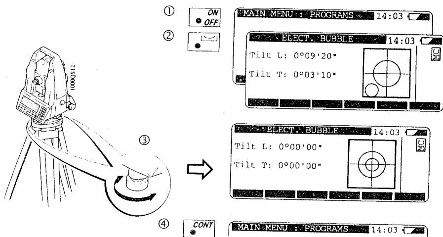
**The instrument can be leveled up using the footscrews,
